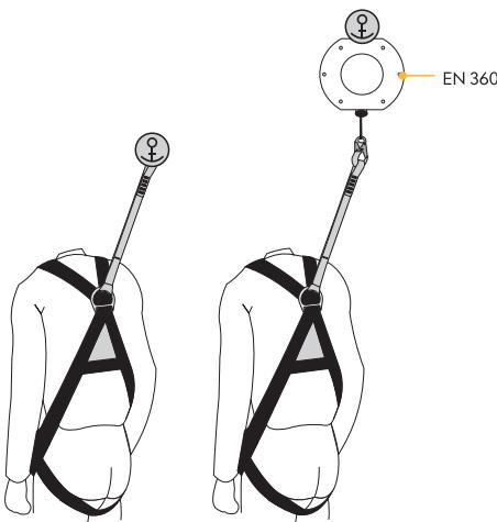
**MBS (Minimum Breaking Strength) = 22 kN**
