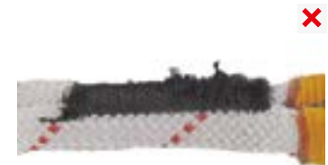
damaged strength seam
