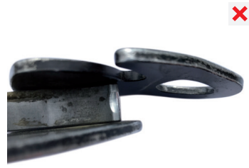
fall arrester body deformation
