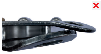
fall arrester body deformation
