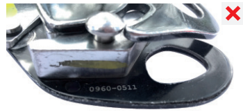
fall arrester body deformation
