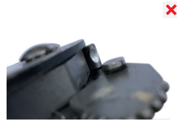
loss of material on fixed part of body
