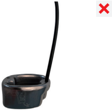
broken wire of the belay device
