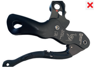
damaged regulation handle
